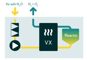
Nitrous oxide in the exhaled air entering the MDU is purified to a degree of over 99 % with the use of the catalytic process in the reactor that breaks down the environmental aggressive nitrous oxide into nitrogen (N2) and oxygen (O2) which are the main constituents of air and can therefore safely be returned to the environment.
